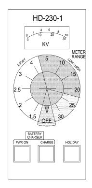
The HD-230-1 Holiday Detector is a safe, rugged but lightweight instrument with a wide range of voltage output, 1.5 - 30kv, making it suitable for use with both thin film Epoxy Powder Coatings or with thicker Polyethylene or Reinforced Coal Tar and Bitumen Coatings.
